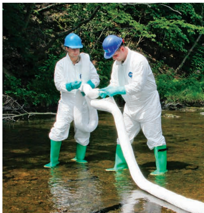
Use connectors to create containment systems big enough to handle almost any size spill.
